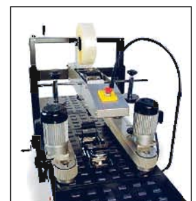
Model CT-75 uses 3" (72mm) Tape Heads
