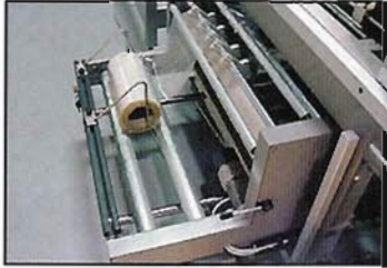
Easy Load Film Cradle with pin wheel hole punch-slides out to change roll, slides back underneath machine out of the way when not in use.
