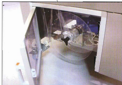
Automatic scrap wind up wheel with built in alarm when full.
