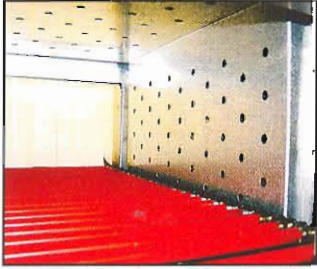
Fully re-circulating air chamber with live roller conveyor.
