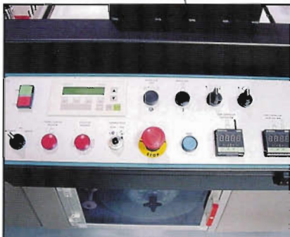
Siemens PLC Controller with 30 product memory functions and built-in self diagnostics
